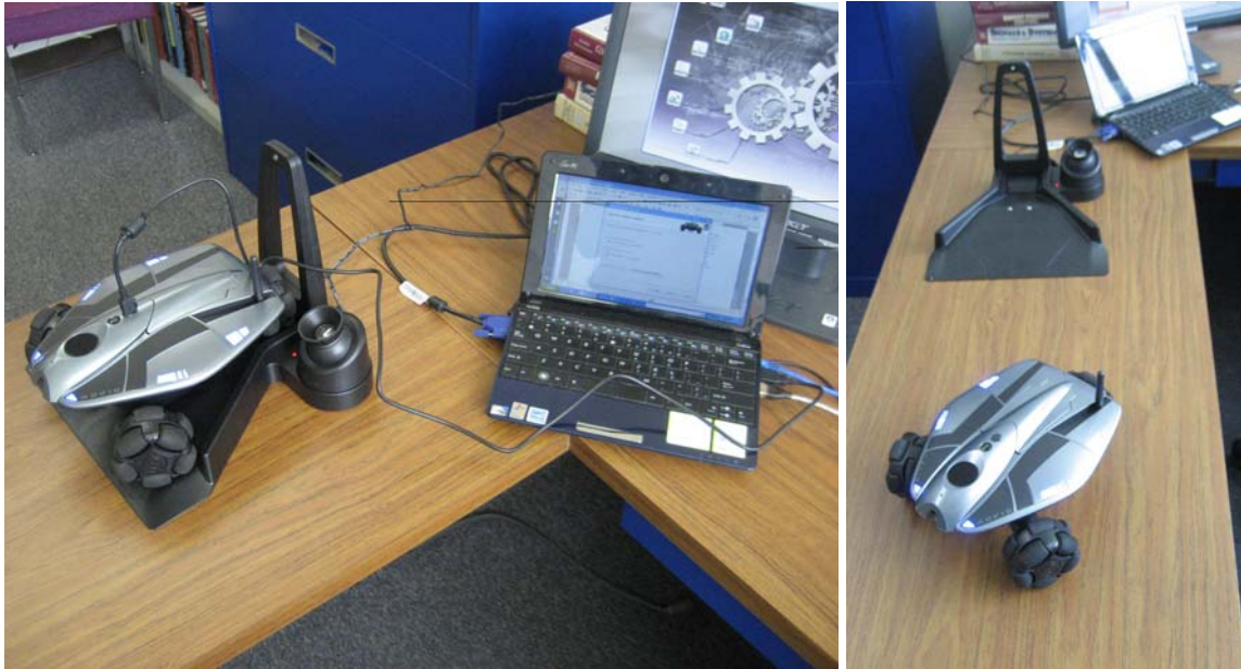
Figure 1. The Rovio wifi-enabled webcam robot. At left: The robot is docked at its power charging station and connected directly to a laptop, to set up wireless connectivity. At right: The robot is on the move! The navigation beacon is the ball-shaped object attached at the side of the docking station. The beacon projects two infrared spots onto the ceiling, which the robot uses to triangulate its position and orientation in a room.
